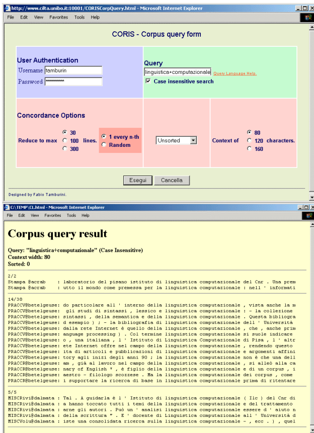
Figure 2: Distributed corpus querying. Note that the concordances belong to the three different computational nodes involved in the Grid (namely, Acrab, Betelgeuse and Dalmata).
